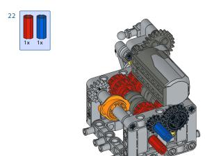
Blue axle joiner marks the transmission's input. Red axle joiner marks the transmission's output. Both input and output are two-sided: you can use them on either side of the transmission (that means, also on the side that is "north" in the picture above).
